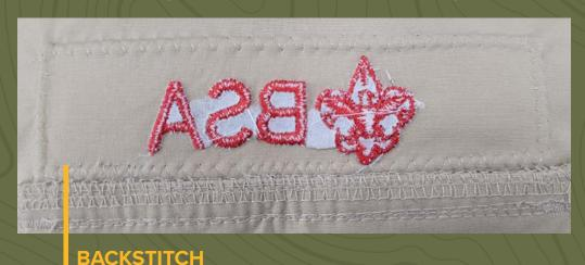
Lots of puckering on the edges. Fabric is pulling. Tension on sewing machine was too high, it is stitching tighter than needed. Tension needs to be dialed down.
